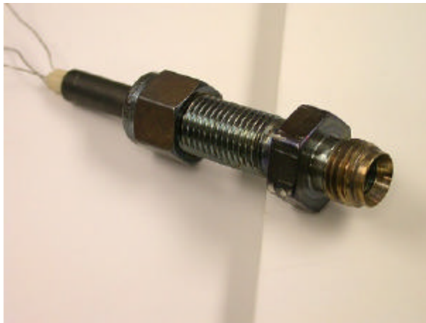
Figure 7: SiC high temperature pressure sensor developed by Sienna Technologies and NASA Glenn Research Center.
